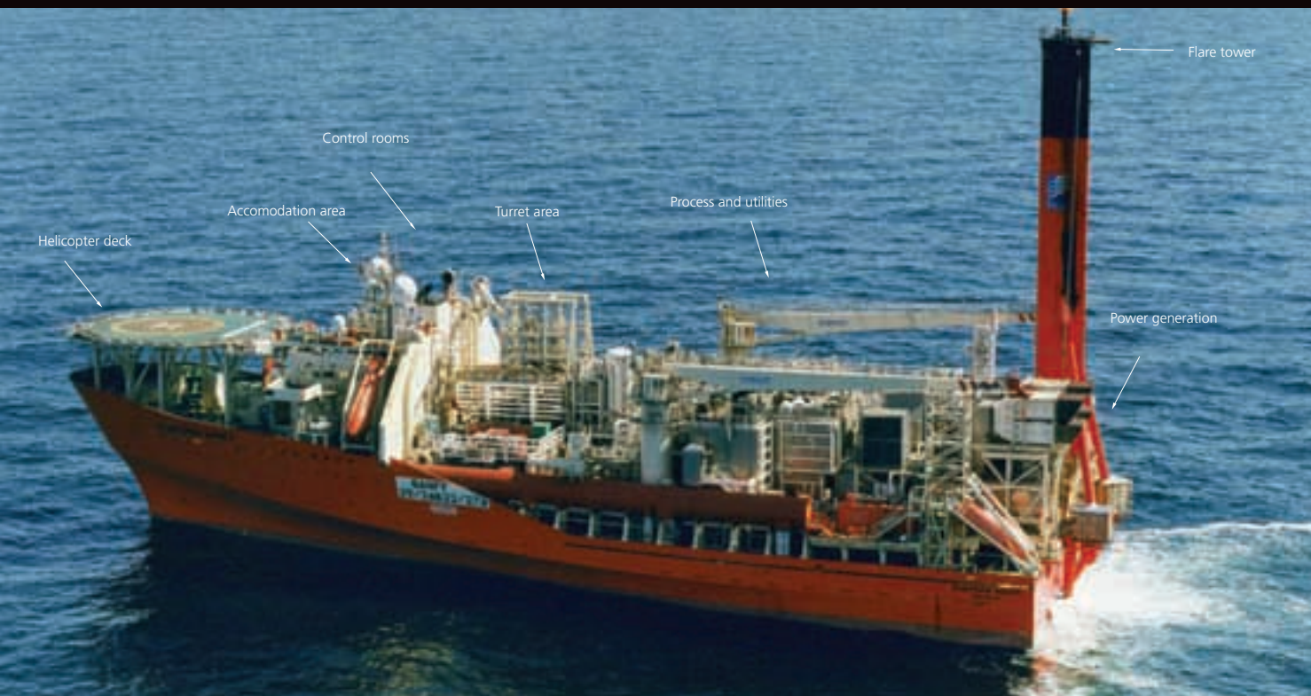
Picture showing main layout of the FPSO.
